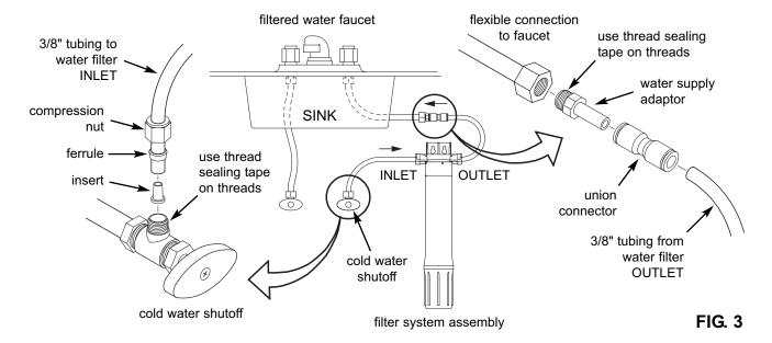
Step B - Make Tubing Connections
